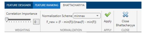
**Apply** updates the ranking display with the new results, displayed along with the original T-Test results.
