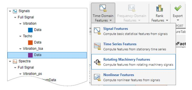
The **Rotating Machinery Features** tab can create features from TSA signals as well as from TSA difference signals and TSA regular signals. Since you have only a TSA signal, the app disables the selections that do require a different signal type.
