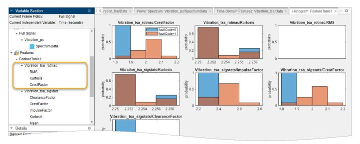
The app automatically adds the new features to the feature table and the **Select Features** list, and plots the new histograms at the top of the histogram display. CrestFactor and Kurtosis histograms are essentially the same whether they are computed as signal features or rotating machinery features, since both computations use the TSA signal as a source.
