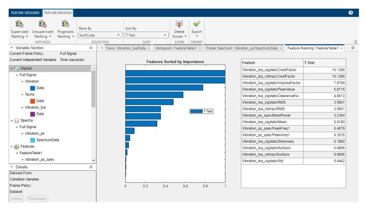
The bar chart legend shows that the initial ranking is performed using the T-Test method. The chart is normalized to 1 to facilitate visual comparison, while the table displays unnormalized ranking scores. The highest ranking feature is CrestFactor, which has the same value whether it was computed as a signal feature or a rotating machinery feature.
