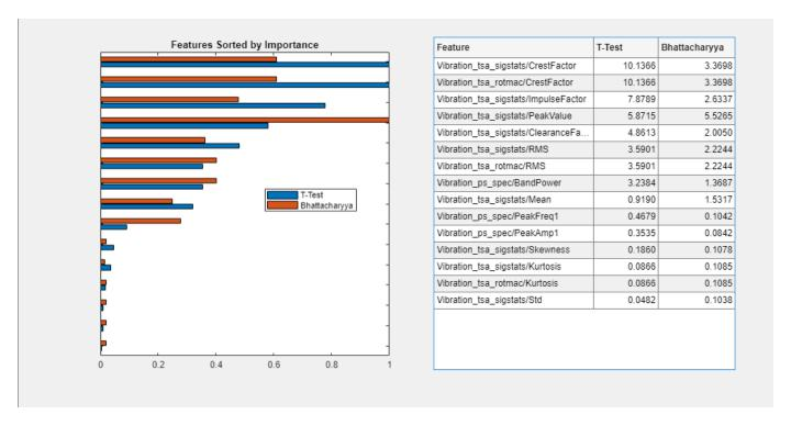
The Bhattacharyya method yields results that are similar to, but not identical to, the T-Test results. The highest ranking feature is PeakValue from the Signal Statistics set. This feature is fourth in the T-test ranking. The crest factor features are still in the top three.
